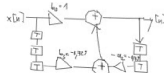
$$y[n] = b_0 \cdot x[n] + b_3 \cdot x[n-3] - a_2 \cdot y[n-2] \quad | \geq$$
